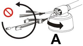
Keep cables from twisting while turning Turn until no threads are exposed.
